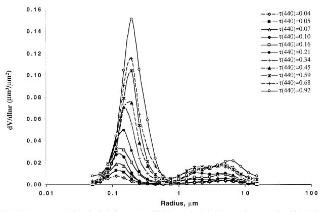
Fig. 2. The average aerosol volume size distribution retrieved at GSFC for aerosol optical thickness at 440 nm varying from 0.04 to 0.92. The aerosol size distributions were derived from the measurements of AERONET ground-based radiometers for 1993–2000 time period.
